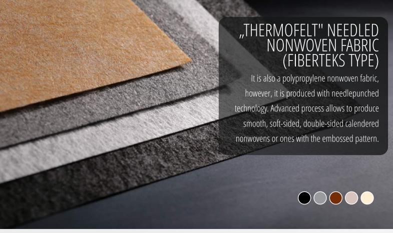
Thermofelt is characterized by its tensile and tearing strength and air permeability. It has hygienic certificates, is flame-retardant, and can also be in fully non-flammable version.
